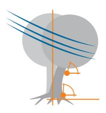
A base sensor measures the root plate inclination directly at the base of the trunk. A control sensor measures the inclination at a height of 2 to 3 metres so that the real wind reaction of the tree can be distinguished from sources of interference.
